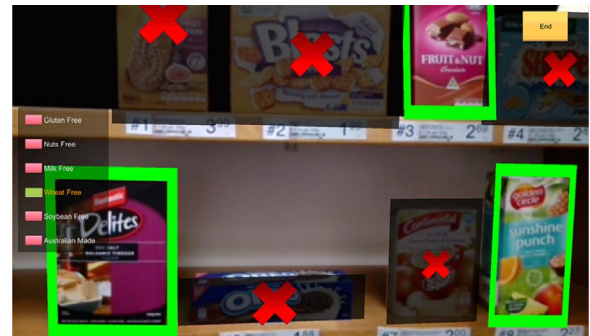
Fig. 2. Example of Filtering visual representation, by highlighting the product of choice with a green enclosing rectangle while hiding the unwanted products with a semi-transparent black object with a red "x" overlay. (For interpretation of the references to color in this figure caption, the reader is referred to the web version of this paper.)
