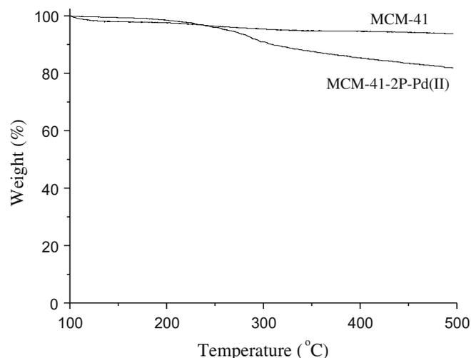
Fig. 1. TGA curves of MCM-41 and MCM-41-2P-Pd(II).
