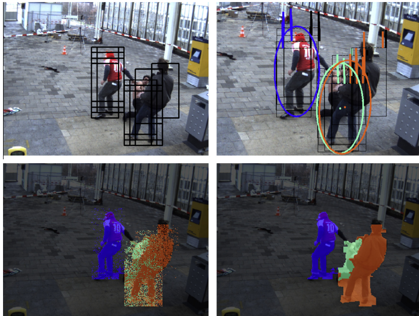
Fig. 1. Best viewed in color. Top left: example illustrating the challenges we address: detections (shown as black boxes) are inaccurate due to challenging poses, perspective and occlusions. Top right: inferred object presence and location. For each detection window the proportion of pixels associated with an object ID is indicated by a color-coded bar graph on top, black bars indicate background. Bottom left: for each pixel we sample an ID to illustrate the mixing proportions (optional post-processing). Bottom right: per pixel object IDs after global image segmentation (optional post-processing). (For interpretation of the references to color in this figure legend, the reader is referred to the web version of this article.)
