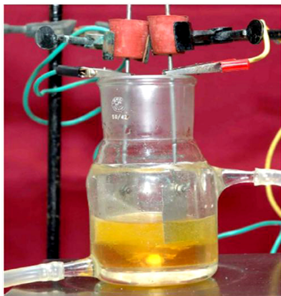
Fig. 1. Electrochemical cell for galvanostatic biphasic electrolytic oxidation.
