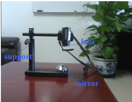
Fig. 1. A catadioptric camera consisting of a quadric mirror and a perspective camera lens: before using this camera, alignment is needed to make the mirror face the lens rightly.
