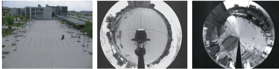
Fig. 1. Examples of images taken with a standard camera (left), hyper-catadioptric camera (center) and with conical mirror camera system (right).
