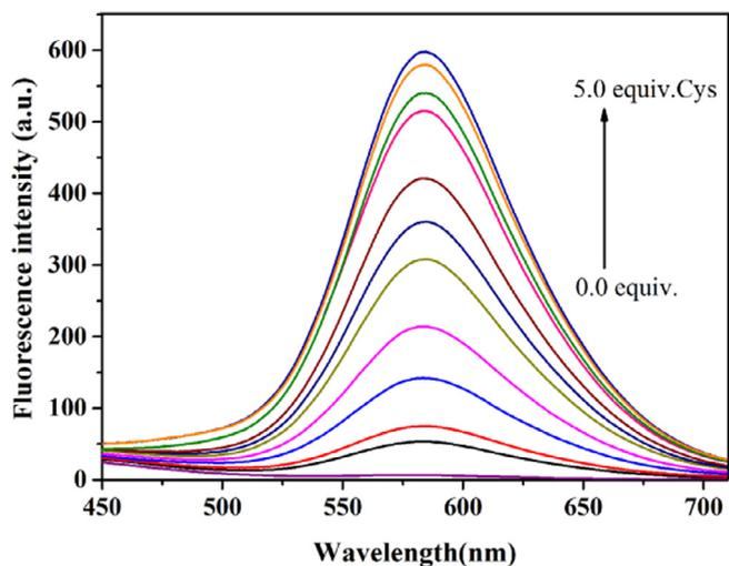
**Fig. 1.** Fluorescent spectra of Probe 1 (5.0  $\mu\text{M}$ ) treated with different concentrations of Cys (0.0–5.0 equiv.) in PBS buffer (10.0 mM, pH 7.4, 1.0 mM CTAB). Spectra were obtained after incubation for 20 min and the excitation wavelength was 368 nm.
