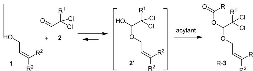
**Scheme 3.** Locking the reversible addition of alcohol **1** and aldehyde **2** through the use of a locking auxiliary.
