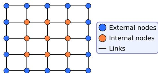
Fig. 1. A  $5 \times 5$  example mesh.
