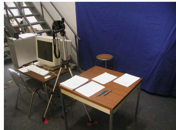
Fig. 2. Setup for the high resolution image capture. Subjects were seated in front of a blue background and recorded using a Canon EOS 10D camera with a Macro Ring Lite MR-14EX ring flash.
