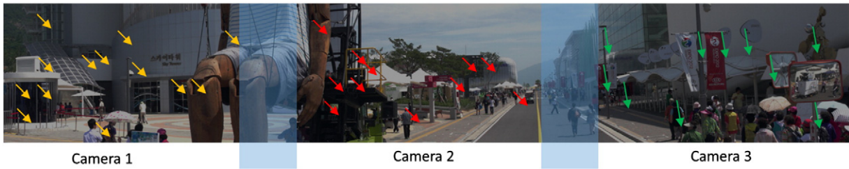
Fig. 1. Stitched frame from a three camera panoramic video. The base of the arrows corresponds to a few salient features in the scene. The yellow, red and green lines illustrate the motion of the tracked features extracted from camera 1, camera 2 and camera 3 respectively at a particular time instance. The figure illustrates that content captured from different cameras may exhibit different motion. This motion is because of the independent motion of each camera and not because of moving objects.
