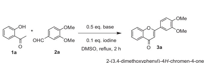
Scheme 2. Reaction of 2'-hydroxyacetophenone with 3,4-dimethoxybenzaldehyde.
