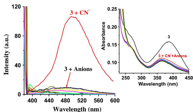
Figure 1. Emission spectra of **3** ( $10\ \mu M$ ) upon addition of different anions (100 equiv) in aqueous medium. Inset: Interference absorption spectra upon the addition of different anions (100 equiv) to a solution of  $3-CN^-$ .
