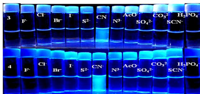
Figure 2. Fluorimetric color changes of **3** and **4** ( $10\ \mu M$ ) with different anions (0–100 equiv) in aqueous medium.
