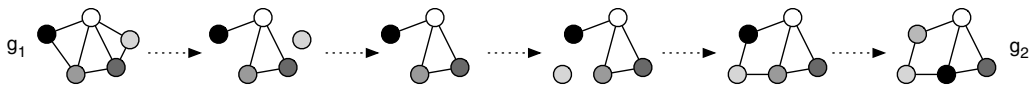
Fig. 1. A possible edit path between graph g_1 and g_2 (node labels are represented by different shades of grey).
