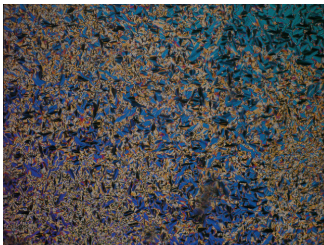
Figure 1. Optical micrograph of 4IM6TP at 170 °C on cooling from the isotropic liquid (crossed polarizer, magnification 200 \times ).
