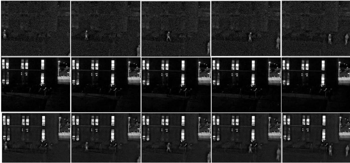
Fig. 1. Illustration of video fusion for scene surveillance. The first and second rows illustrate several frames from an infrared and a visible light video, respectively, both capturing the same scene. The last row illustrates the corresponding frames from the fused video, which is obtained by our proposed method. As shown in the last row, the background images (extracted from the visible light video) and the moving targets (extracted from the infrared video) are well-integrated in the fused video. Moreover, the noise is also suppressed during the fusion process.
