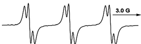
Figure 1. EPR spectrum of PINO obtained by mixing NHPI (0.01 M) with m -CPBA (0.01 M) in \text{CH}_3\text{CN} at room temperature.
