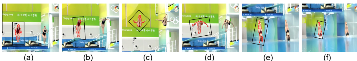
Fig. 1. Simultaneously tracking and segmentation of non-rigid object using our method. In tracking, a bounding box (black) is obtained by image warping with translation and rotation. In segmentation, a contour (red) is calculated by level-set evolution. The size of the bounding box is slightly updated to make it tighter to the target object. (For interpretation of the references to color in this figure legend, the reader is referred to the web version of this article.)
