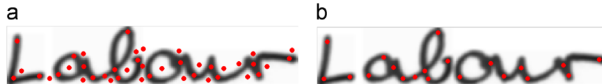
Fig. 1. Keypoints selection and the corresponding triangular mesh structure. (a) Keypoints detected by SIFT detector. (b) Removing uninteresting points. (For interpretation of the references to color in this figure caption, the reader is referred to the web version of this paper.)
