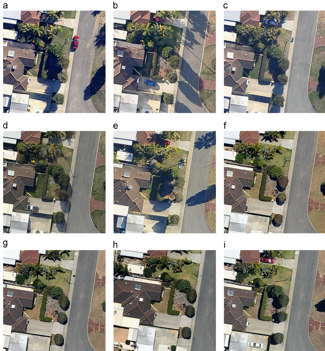
Fig. 1. Input images to our algorithm (for easier visualization, only 400 \times 400 pixel sub-regions of 1500 \times 1500 pixel images used as an actual input are shown). These correspond to approximately the same land area imaged from an aeroplane on different days and at different times of the day, and registered using a state-of-the-art commercial registration system which uses both GPS and image data. Notice that despite the registration substantial registration errors remain (compare images (h) and (i), for example – the misalignment error between them is 78 pixels, Sections 3.1 and 3.3 for details). Also, observe the extent and the nature of appearance changes across images: cars move in and out, shadows change in their shape, direction, and intensity, grass and leaves change color across seasons.
