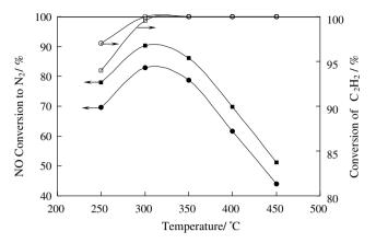
**Fig. 1.** NO conversion to N<sub>2</sub> (close symbols) and conversion of  $C_2H_2$  (open symbols) in  $C_2H_2$ -SCR as a function of temperature over HFER  $(\bullet, \bigcirc)$  and 2%Zr/HFER  $(\blacksquare, \bigcirc)$ .
