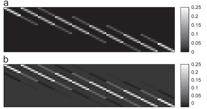
Fig. 1. The projection matrix \mathbf{P} \in \mathbb{R}^{25 \times 100} modelling the process of downsampling a 10 \times 10 pixel image to 5 \times 5 pixels, using (a) bilinear and (b) bicubic projection models, shown as an image. For the interpretation of image intensities see the associated grey level scales on the right.
