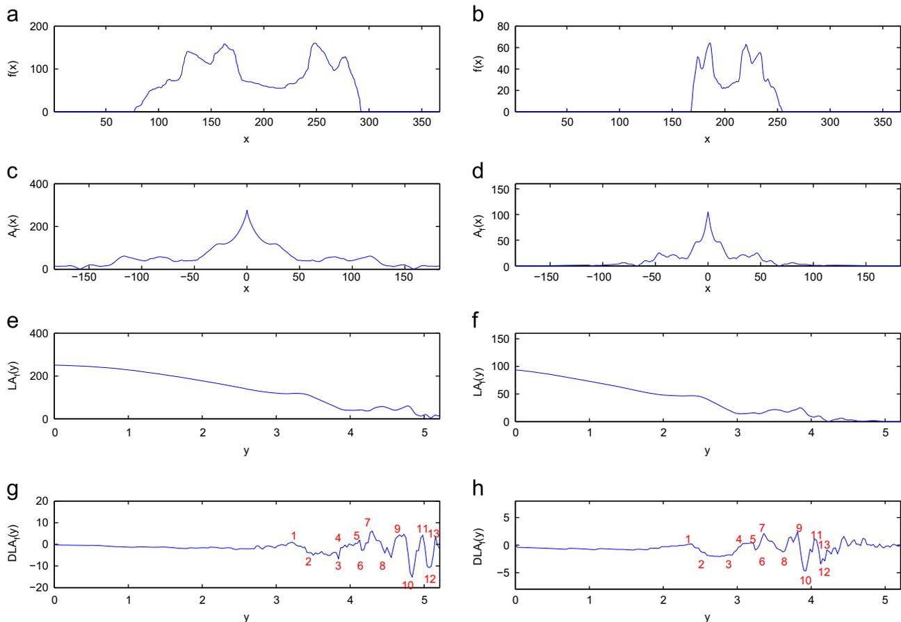
Fig. 4. (a) and (b) respectively original 1d signals from the Radon domain (a column of Fig. 3(a)) for  $\theta = 0$ , and  $\theta = 120$ . (c) and (d) Amplitude-extracted signals  $A_f(y)$  and  $A_g(y)$  respectively. (e) and (f) Results of the log-mapping  $\mathcal{L}A_f(y)$  and  $\mathcal{L}A_g(y)$  respectively from the half domain (c) and (d) ( $\alpha \geq 1$ ). (g) and (h) Results of the differentiation  $D\mathcal{L}A_f(y)$  and  $D\mathcal{L}A_g(y)$  respectively.
