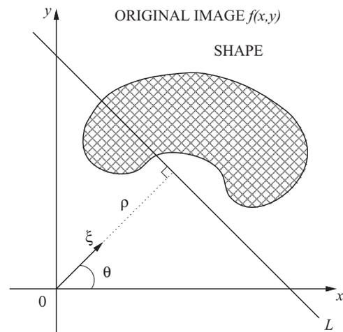
Fig. 1. Graphical illustration of the Radon transform.
