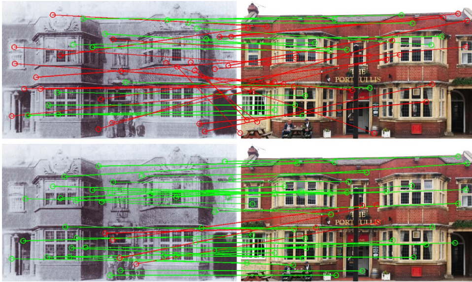
Fig. 1. An example of image matching. Top: the GNCCP algorithm [6] without using symmetry constraints. Bottom: the same algorithm boosted by our symmetry integration strategy. Green and red lines indicate respectively correct and wrong matches – same patterns are used for Figs. 6–8 and are best viewed in color. (For interpretation of the references to color in this figure caption, the reader is referred to the web version of this paper.)
