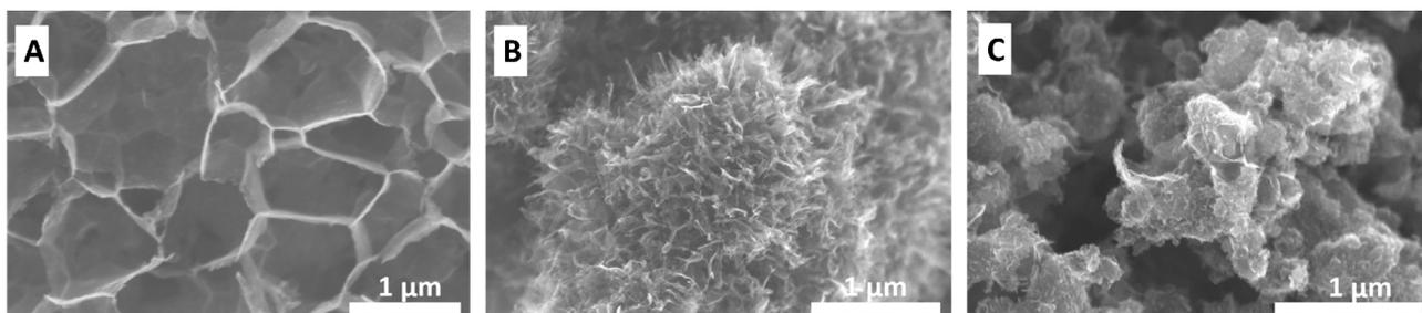
**Fig. 3.** FESEM images of graphene synthesized from CO reaction with (a) 10  $\mu\text{m}$   $\text{Li}_2\text{O}$  particles, (b) 1  $\mu\text{m}$   $\text{Li}_2\text{O}$  particles, and (c) 0.4  $\mu\text{m}$   $\text{Li}_2\text{O}$  particles.
