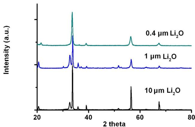
**Fig. 2.** XRD patterns of  $\text{Li}_2\text{O}$  with various particle sizes.
