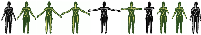
Fig. 1. Gesture representation from key poses: our method represents a body gesture as a sequence of a few extreme body poses, referred to as key poses . In the example above, a gesture composed by opening arms and then clapping hands is represented by the key poses in black.
