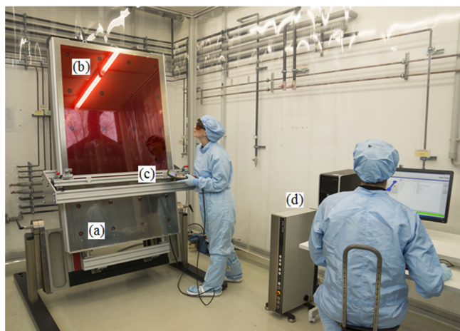
Fig. 1. The proposed wiping-coating device in order to coat large area substrates: (a) aluminum plate with holes connected to the vacuum pumps; (b) polycarbonate plate; (c) sol tank with adjustable speed and adjustable distance from the substrate; (d) processor controllers.
