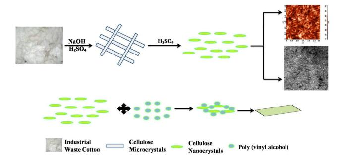
Schematic representation of the preparation of cellulose nanocrystals from industrial waste cotton
