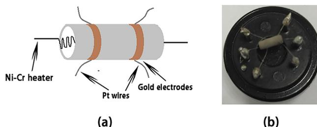
Fig. 1. (a) schematic diagram of the thick film sensor; (b) Fabricated sensor.
