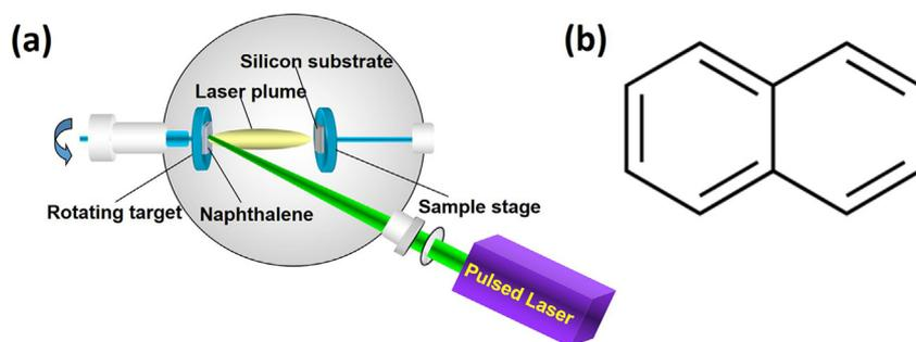
Fig. 1. (a) Schematic diagram of the experimental setup (b) Structural formula of naphthalene.
