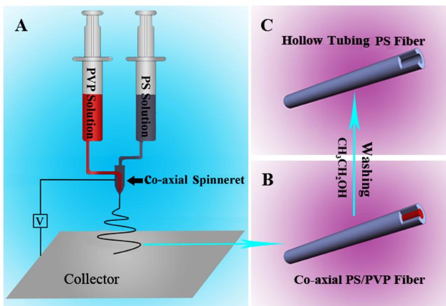
**Fig. 1.** Schematic representation of the synthesis procedure for HF by the co-axial electrospinning.
