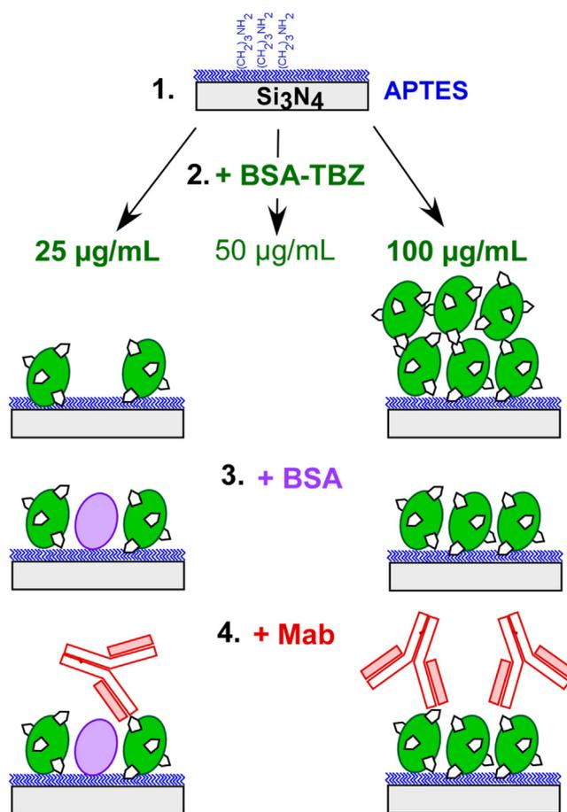
**Fig. 1.** Schematic of the procedure employed for biofunctionalization of  $\text{Si}_3\text{N}_4$  surfaces and subsequent immunoassay for detection of fungicide TBZ.  $\text{Si}_3\text{N}_4$  surfaces were modified with APTES (1), spotted with BSA-TBZ conjugate (probe) using solutions with different concentrations (25, 50 and 100  $\mu\text{g/mL}$ ) (2), blocked with BSA (3), and exposed to a solution of monoclonal antibody against TBZ (Mab) (4).
