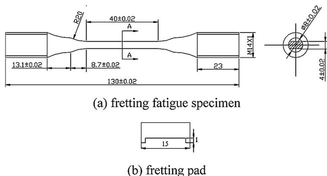
Fig. 1. Schematic drawing of FF specimens and fretting pads.
