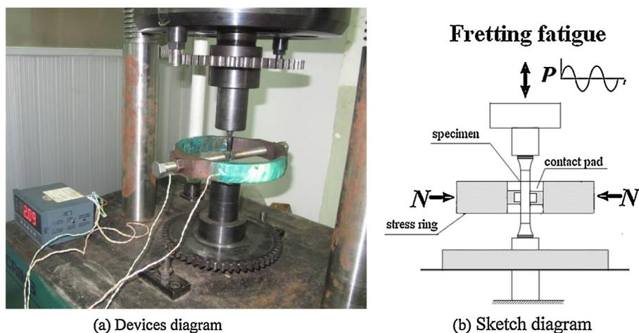
Fig. 2. Devices and sketch diagram of fretting fatigue test.
