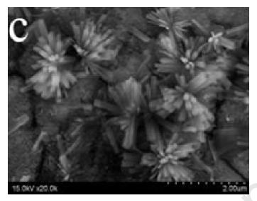
Unique ZnSe nanoflowers have been successfully synthesized by reaction of Se powder with Zn substrates.>> Characterized by XRD, SEM, TEM, XPS, EDS and Raman spectroscopy .>> Were single crystals with cubic zinc blende (ZB) structure>>Have excellent field emission properties and optical properties.
