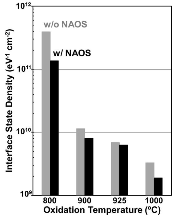
**Fig. 2.** Interface state density for the <Al/SiO<sub>2</sub>/n-Si(100)> MOS structure with and without the NAOS treatment vs. the thermal oxidation temperature.
