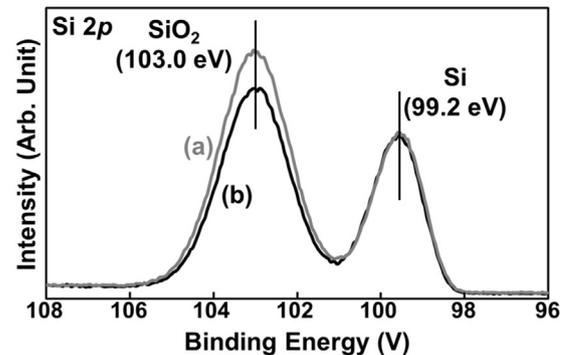
**Fig. 3.** XPS spectra of the SiO<sub>2</sub>/n-Si(100) structure after thermal oxidation at 925 °C: a) without the NAOS treatment; b) with the NAOS treatment performed before thermal oxidation.
