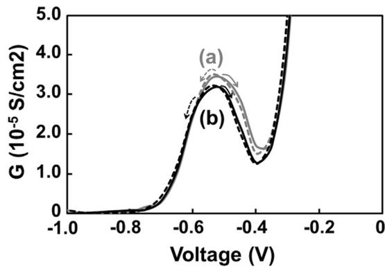
**Fig. 1.** G-V curves at 10 kHz for the <Al/SiO<sub>2</sub>/n-Si(100)> structure after thermal oxidation at 925 °C: a) without the NAOS treatment, b) with the NAOS treatment performed before thermal oxidation. The solid and dotted lines indicate G-V curves measured during forward and reverse sweeps, respectively. The arrows indicate the voltage sweep direction.
