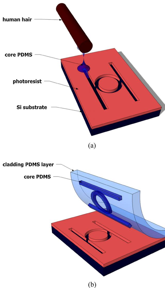
Fig. 1. a) Illustration of channel filling with PDMS for the ring resonator structure preparation and b) illustration of mechanical separation of cured PDMS ring resonator.
