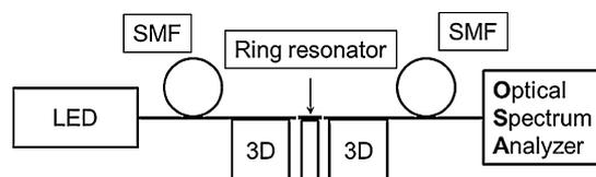
Fig. 2. Experimental stage for the spectral characterization of PDMS waveguide structures, LED – light emitting diode, SMF – single-mode optical fiber, 3D – nanostaging mechanical stage.
