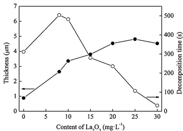
Fig. 2. Thickness of Ni–P–La coating and decomposition time of electrolyte under different content of  $\text{La}_2\text{O}_3$  in electrolyte.
