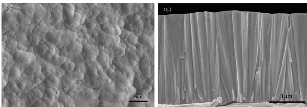
Fig. 1. (a) Surface morphology and (b) cross section of Ni–P–La coating ( $10 \text{ mg L}^{-1} \text{ La}_2\text{O}_3$ ).
