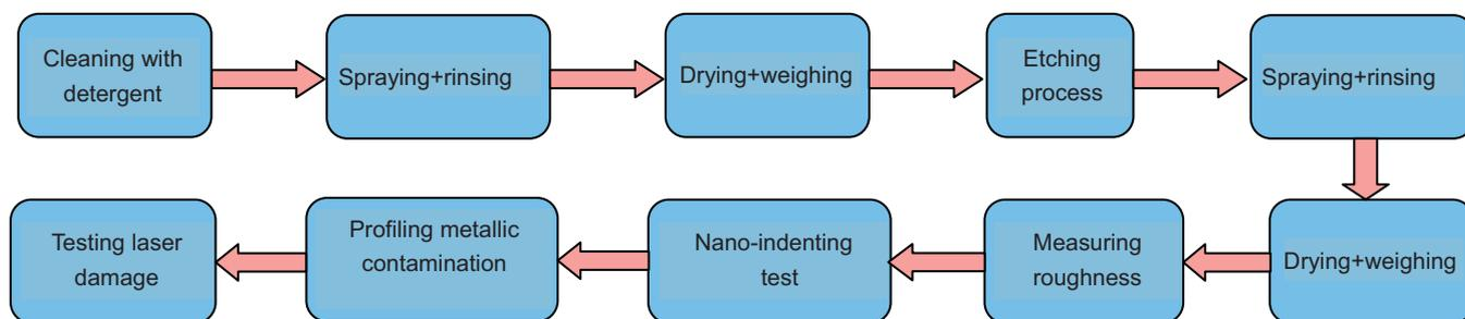
Fig. 1. Flowchart of experimental procedure. Each sample was immersed in a specific solution for a certain time.
