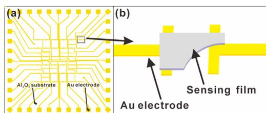
**Fig. 1.** (a) Schematic diagram of test chip. (b) Configuration of sensing film and Au electrode.
