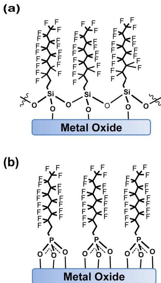
Fig. 1. Schematic illustration of the formation of self-assembled monolayers of HDF-PA and HDF-S on  $\text{Al}_2\text{O}_3$  thin films.
