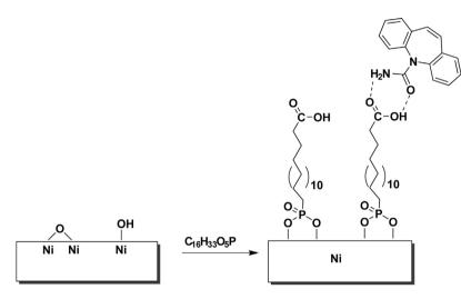
Fig. 2. Addition of COOH-PA SAM on NiO metal substrate and interaction with CBZ. Orientation of SAMs is consistent between NiO and ZnO metal substrates.
