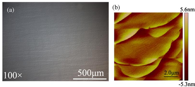
Fig. 1. Initial surface of Ga-face (0001) GaN wafer. (a) Microscope image (b) AFM image.
