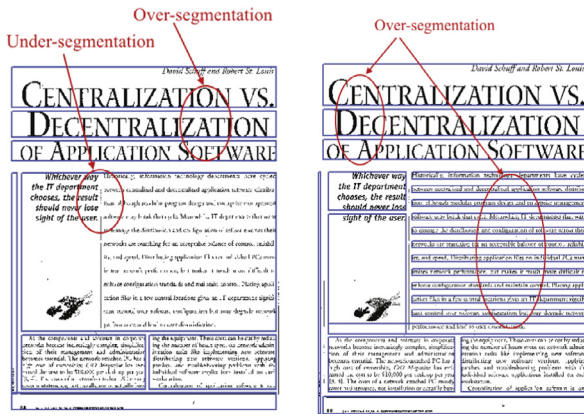
Fig. 1. Illustration of under-segmentation and over-segmentation errors.
