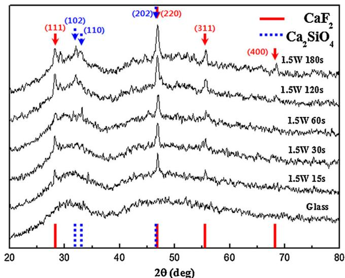
Fig. 1. XRD patterns of the glass and glass-ceramics prepared by space-selective CO<sub>2</sub> laser annealing with various exposure times.
