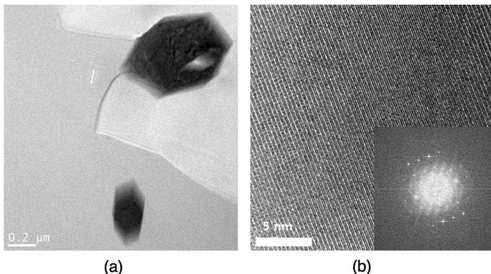
Fig. 2. (a) TEM micrograph of crystallites, and (b) high-resolution image of crystalline area in the Er/Yb co-doped glass-ceramics (insert shows its Fourier transform) precipitated by exposure to CO<sub>2</sub> laser for 3 min.
