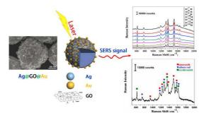
The GO embedded sandwich nanoparticles are capable of serving as an ultrasensitive, highly reproducible and stable SERS platform.
