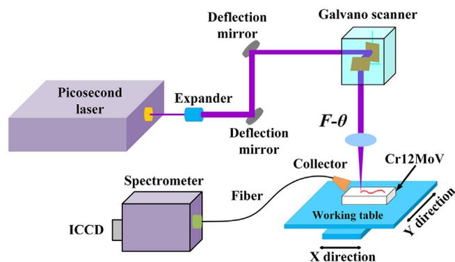
**Fig. 1.** Schematic diagram of experimental setup for picosecond laser ablation of Cr12MoV.
