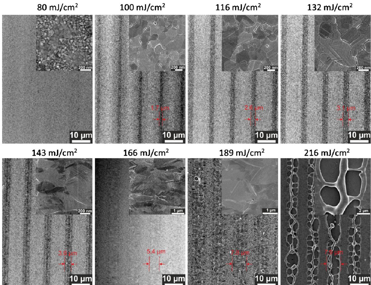
Fig. 2. SEM images of the morphology after masked laser annealing with 2 pulses at different fluences. The insets are magnified SEM images of the corresponding annealed areas.
