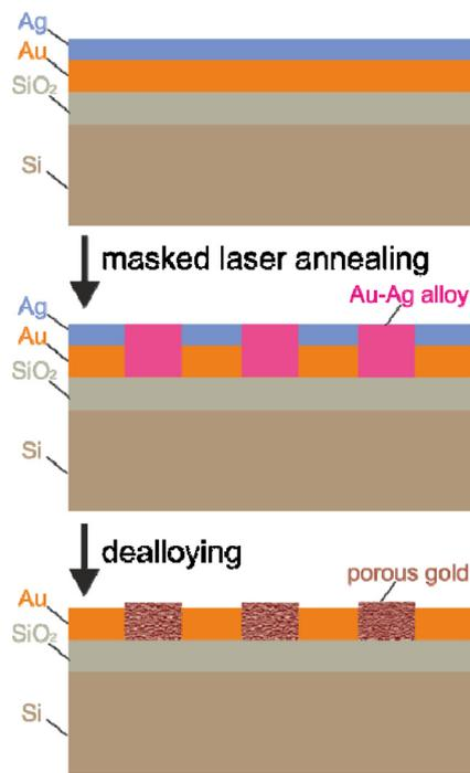
Fig. 1. Schematic of the fabrication of the complex patterned gold structures.
