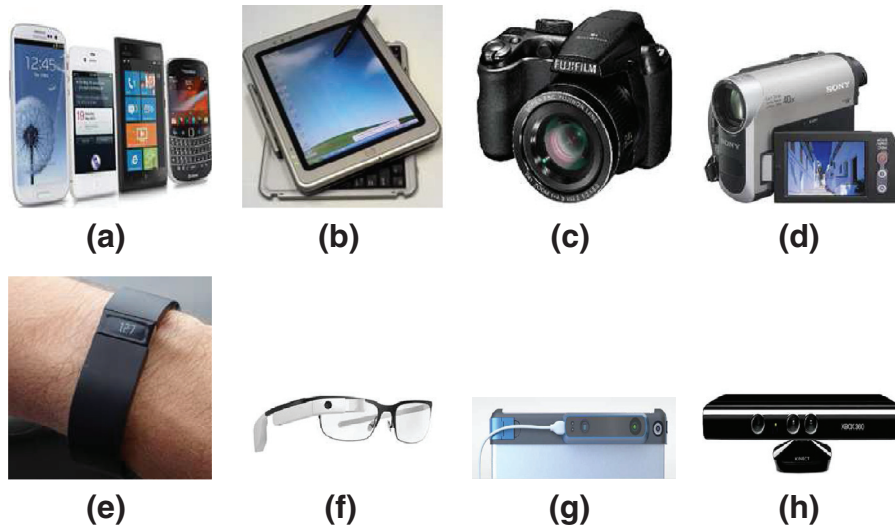
Fig. 1. Examples of mobile devices capable of capturing biometric data: (a) smartphones, (b) tablet computers, (c) digital cameras, (d) digital video recorders, (e) wearable activity trackers (e.g., Fitbit), (f) wearable head-mount displays (e.g., Google Glass), (g) 3D sensors (e.g., [14]), and (h) portable game consoles (e.g., XBOX Kinect).
