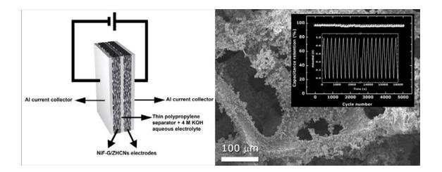
The fabricated symmetric supercapacitor based on NiF-G/ZHCNs as the negative and positive electrodes exhibited a specific areal capacitance of 222 mF cm<sup>-2</sup> at 1.0 mA cm<sup>-2</sup> and 96% specific capacitance retention after 5000 cycles. These results showed that electrical and ionic conductivities of the NiF-G/ZHCNs are suitable for symmetric supercapacitor application.
