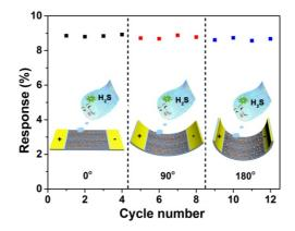
Stable response of SWNT-Fe $_2$ O $_3$  composite film gas sensors under different bending angles upon exposure to 20 ppm  $H_2$ S
